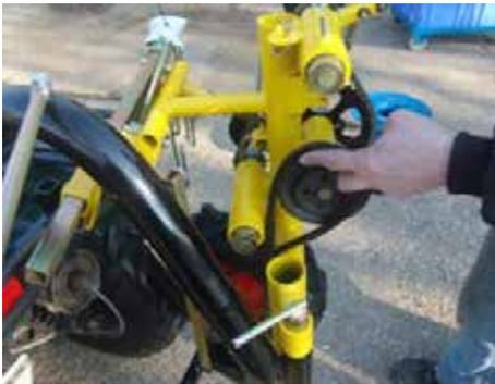
3. Pull the winder away from the bike and tension the belt by attaching the stay bar from the wheel arm to the winder and securing with the yellow knob.
