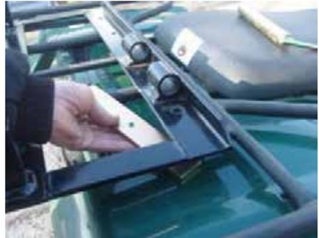
4. Attach the winder to the wheel arm using the connection pin ensuring the reel shaft is on top of the machine. Swing into working position. Rotate the winder fully to check that there is clearance on all moving parts between the winder and the ATV.
