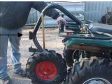
3. Once the required position is reached, secure the mounting frame with the clamping plates and lightly tighten. Try to clamp the mounting frame onto the strongest part of the rack.
