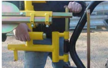
5. Tighten the clamp plate bolts. It may be necessary to trim the ATV mudguard and adjust the position of the rear lights if fitted.
