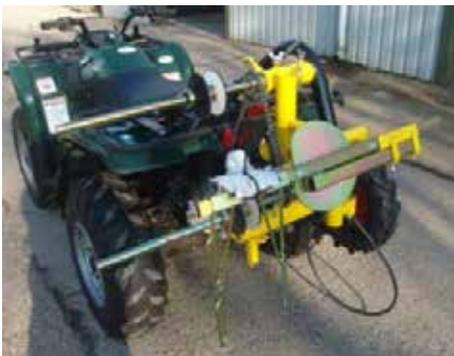
2. Place reels on the reel shafts with springs between and hold
