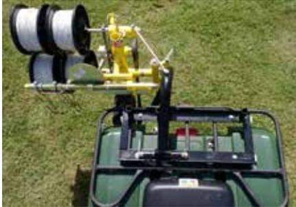
2. Push the winder towards the bike and slip the drive belt over the Top Pulley and Wheel Arm Pulley twisting it to form a figure of eight.
