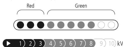
*Note:* If ten Indicator light segments are illuminated, the output voltage may be more than 10 kV (10,000 V).
