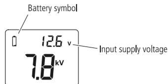
When the voltage is outside the normal range (below 11.8 V or above 17 V), the battery symbol flashes.
