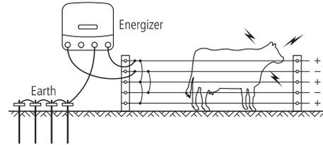
*Note:* The earth monitoring feature cannot be used with a bi-polar installation.
