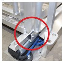
Don't forget to secure it with the linch pin.
