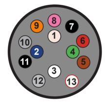
Diagram shows 13 pin wiring as fitted to rear of socket using corresponding numbers and colours shown
