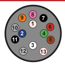
Diagram shows 13 pin wiring as fitted to **rear** of socket using corresponding numbers and colours shown
