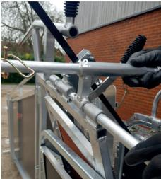
12. Pull the Panel Connector towards the Small Grip -Panel and secure using a Pipe Pin (3). Next Secure the Black Slider located on the RaceGrip Handle to the Small Grip Panel usingPipe Pin (3).
