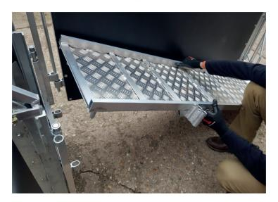
Note: The Entry Ramp must sit on top of the Anti Backing Gate Frame.
