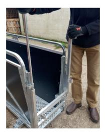
3. Place the Exit Ramp (2) inside the yard race. Secure by locating the connectors onto the Yard Attachment Bracket and locking with a Pipe Pin (3).
