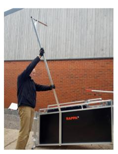
Drenching Pole is fitted onto the yard race and secure with a lynch pin.
