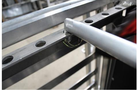
6. Put the weigh head stand into its slot.
