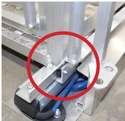
Don't forget to secure it with the linch pin.
