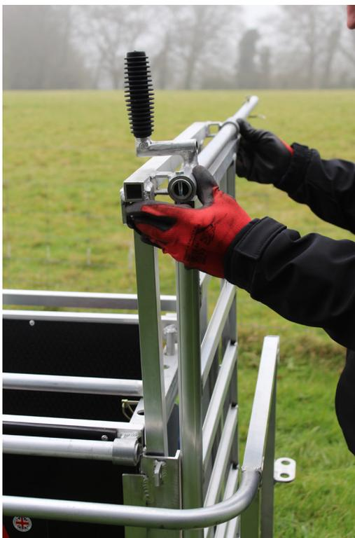
2. Do the same on the opposite side, placing the front exit gate - with the yellow knob on the outside - over the inner frame. Slot inside the gate guide and clip on the linch pin.
